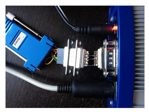
Davis stations datalogger interface comes in two kinds: "standard" datalogger or "APRS" datalogger. According to my current knowledge, both types work fine with WX3in1 Mini (it doesn't use an "APRS" feature of datalogger but "APRS" datalogger has also the same communication options like "standard" one).
